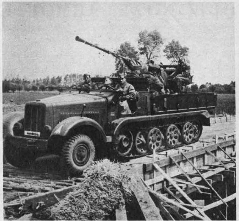
Several types of Nazi AA artillery have been mounted on half-tracks. This long-barreled 37-mm. AA gun is also very effective against tanks. Large overlapping bogie wheels are characteristic of Nazi half-tracks.
